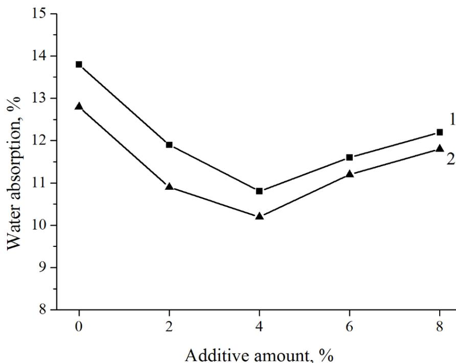
**Figure 3.** Dependences of the water absorption of concrete on the amount of the additives based on calcium hydrosilicates (xonotlite and tobermorite) (1) and wollastonite (2).
