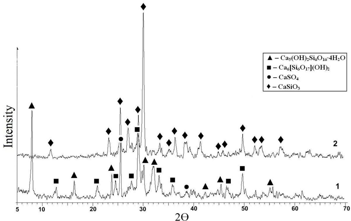
**Figure 1.** Diffractograms of samples obtained as a result of autoclave borogypsum treatment: 1 – initial sample (before annealing); 2 – after annealing at  $1000 \text{ }^\circ\text{C}$ .
