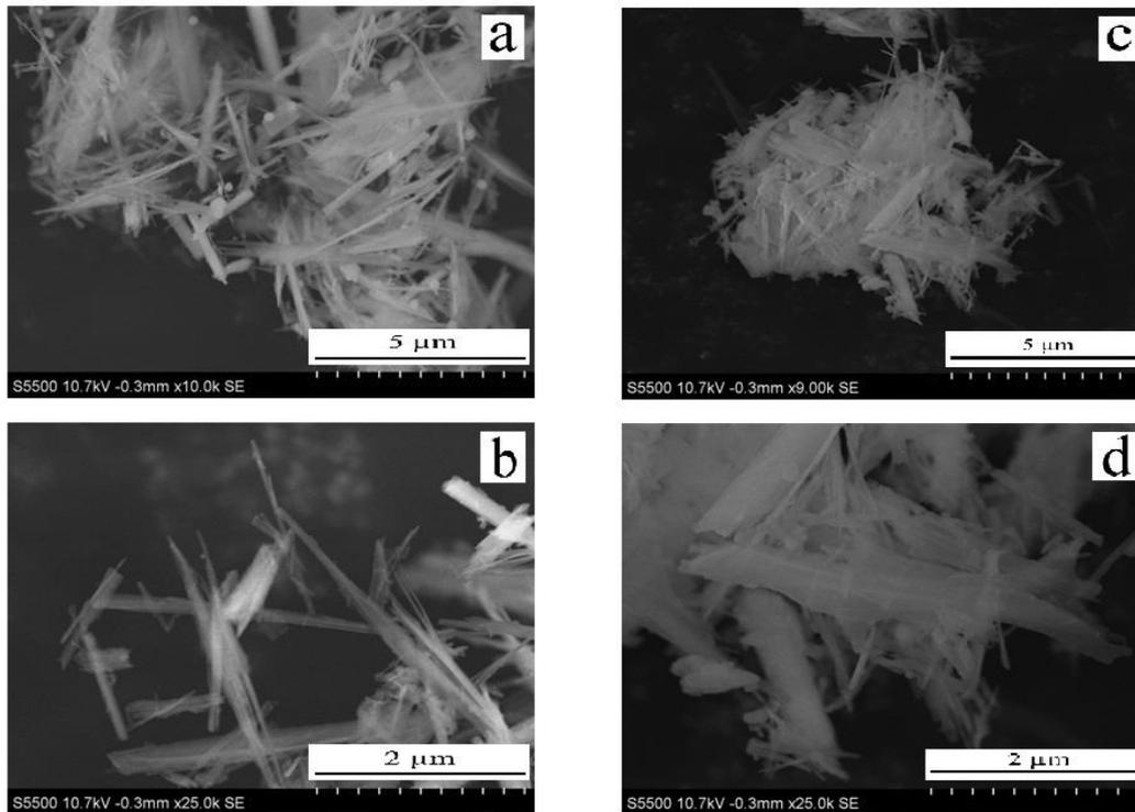
**Figure 2.** SEM images of microparticles of the sample obtained as a result of autoclave synthesis, after drying at 85 °C (a, b) and after annealing at 1000 °C for 1 hour (c, d).
