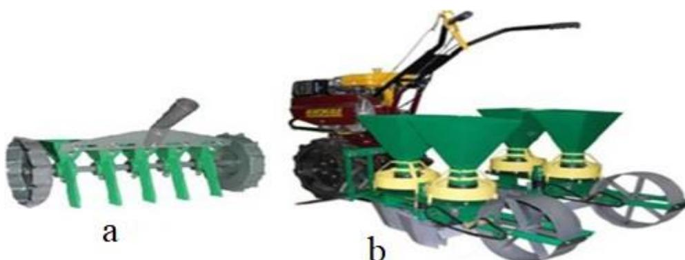
Fig. 6. Sections of "Hatzenbichler" precision seeders
