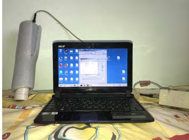
Fig 1: BDKG-03 (Highly sensitive scintillation intelligent gamma detection unit)
