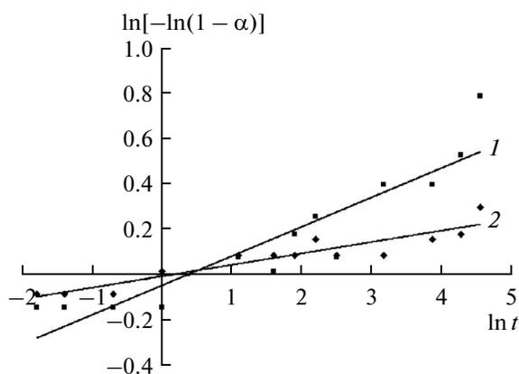
**Fig. 2.** Target product yield degree logarithm  $\ln[-\ln(1-\alpha)]$  versus time logarithm  $\ln t$  for the formation of calcium hydrosilicate under (1) ultrasonic treatment conditions and (2) conventional stirring.
