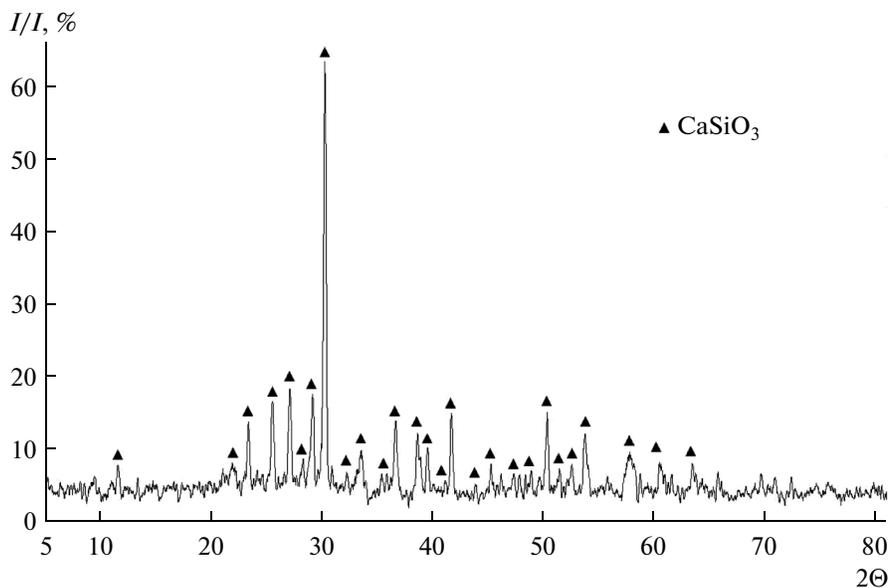
**Fig. 3.** X-ray diffraction pattern of the sample synthesized under ultrasonic treatment conditions for 9 h after annealing at  $1000^\circ\text{C}$  for 40 min.
