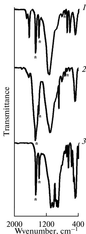
**Fig. 4.** IR spectra of samples: (1) borogypsum (reference sample), (2) synthesized calcium hydrosilicate after drying at 85°C, (3) synthesized calcium hydrosilicate after annealing at 1000°C, (\*) Nujol peaks.
