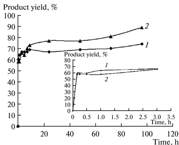
Fig. 1. Target product yield under (1) conventional stirring and (2) ultrasonic treatment versus time.
