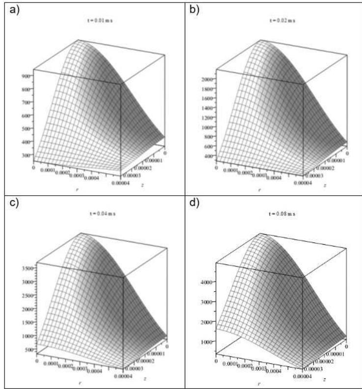
Figure 1. Temperature distribution for pulses of various durations
