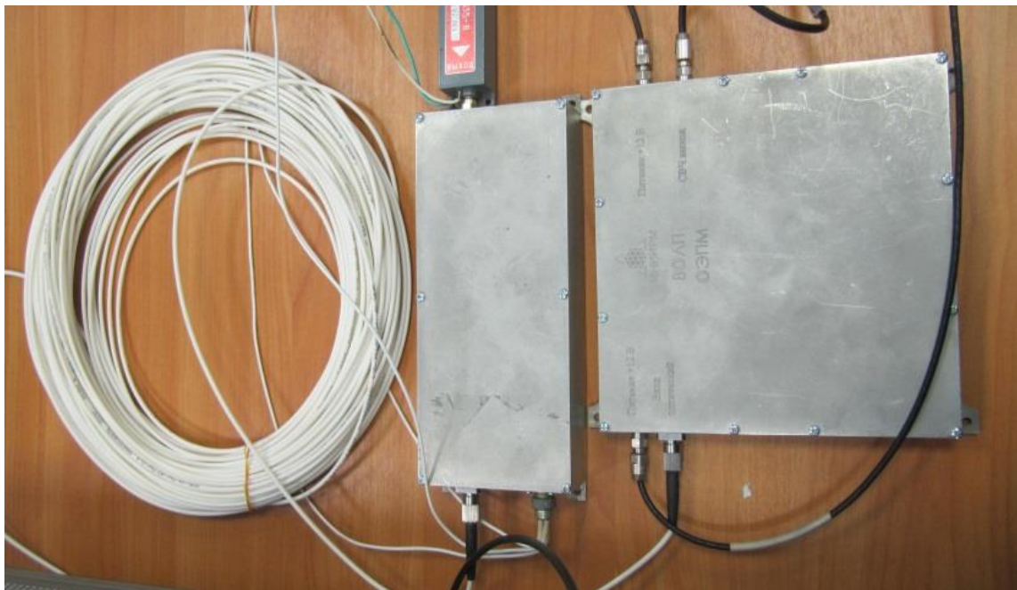
Figure 2. The Fiber-optic communication line for microwave signal transmission in X-band
