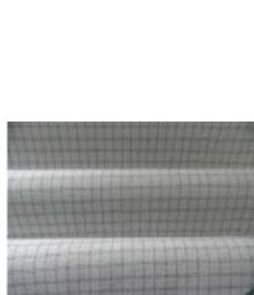
Fig.9. Antistatic fabric with Thermo-Control
