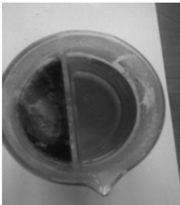
Fig. 6. Co-EDTA solution (separated by a diaphragm, with the cathode being on the left) after the electrochemical process.
