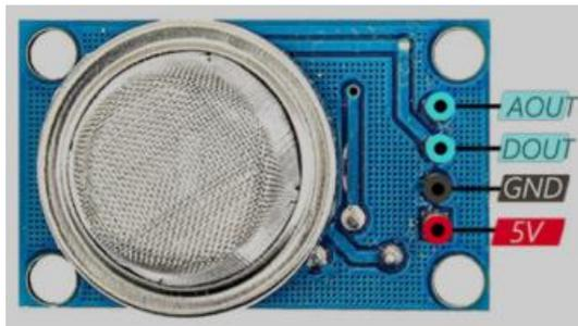
Figure 2 – MQ-4 methane gas sensor
