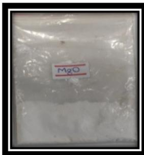
**Fig.6. Final Product Magnesium Oxide Nanoparticles Powder**
