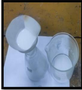
**Fig.4. Washing and Filtration of Magnesium Hydroxide Precipitate**
