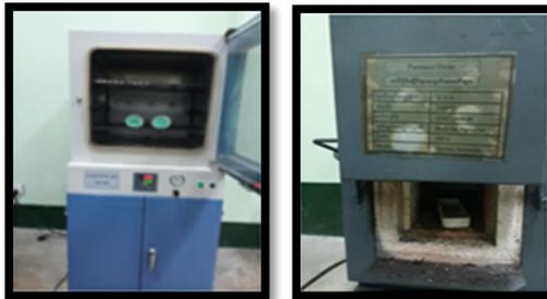
**Fig.5. Drying and Calcination Magnesium Hydroxide Precipitate**
