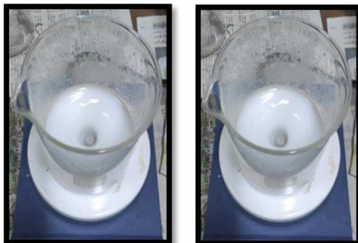
**Fig.3. Precipitation of Magnesium Hydroxide**
