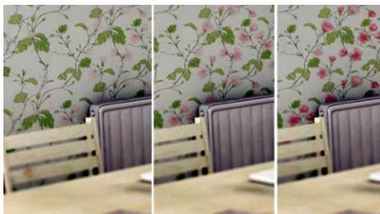
Figure 6. Thermo wallpaper. The pattern “blooms” under the influence of heat from the battery. Available from: https://zen.yandex.ru/media/masterya/sovremennye-materialy-dlia-otdelki-sten-v-kvartire-5c907abb93a05800b39d4a31 [Accessed 5th august 2020].
